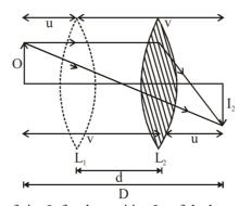
Figure (ii) shows the diminished image of size  $I_2$  for the position  $L_2$  of the lens.
