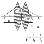
If P is the power of the combination, then  $P = P_1 + P_2$  where  $P_1$  and  $P_2$  are the powers of the individual lenses. If two lenses are separated by distance d then focal length of system of two lenses is given by
